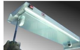
**Step 5:** Attach the reflector using the provided screws and peel off the protective film from its surface.
