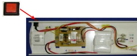
**Step 8:** Activate the electric supply and press the red button to test the lamp
