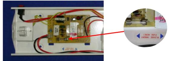
**Step 4:** Install the provided fuse at the fuse holder.
