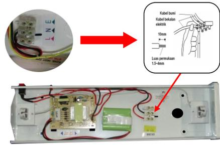
**Step 3:** Connect the supply cable to the provided connector.
