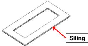
**Step 1:** Prepare ceiling hole according to the given size.
