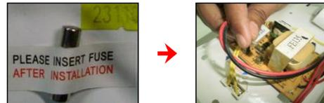
**Step 8:** Detach the fuse from sticker and attach it to its holder after the supply cable is connected
