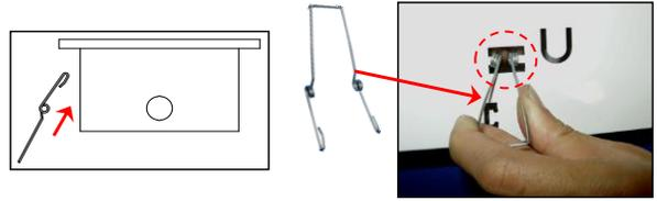
**Step 4:** Insert all the four springs at the respective four sides of lamp frame as shown in the above picture.
