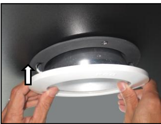
Step 6 : Insert the spring from the lamp cover into the hole on the lamp frame. Make sure that the lamp cover is placed properly.
