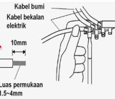
**Step 2:** Connect the supply cable to the terminal block on the chassis.
