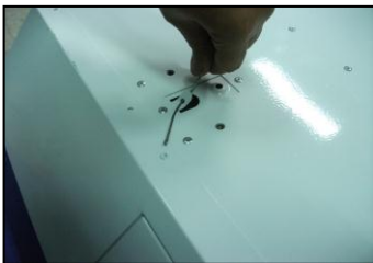
Step 2: Insert suitable wire and twist it for minimum five times as shown in the picture.
