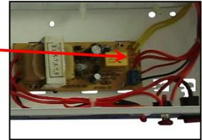
**Step 4:** Install the provided fuse at the fuse holder after connect supply wire.
