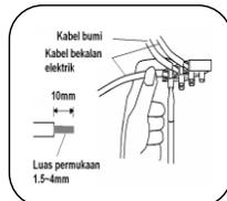
**Step 3:** Connect the supply cable at the prepared connector.
