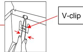
**Step 7:** Make sure that the v-clip is pressed in order to push it inside the v-clip holder.
