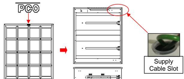
**Step 9:** The illustration shows a lamp frame which is finished installed and the location of PCO logo (Emboss I downward) should be parallel with the supply cable's
