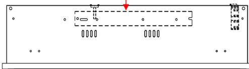
**Step 3:** Replace the ballast if there are any damages recognized and make sure that all the wires are fixed again according to the existing wiring. The wiring diagram on the ballast can be referred for this purpose. Conduct a light test before reattach the louver.
