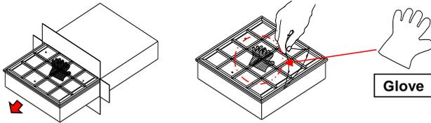
**Step 1:** Take out the lamp frame from the box in a proper way and remove the hand glove from the bottom of the plastic cover.
