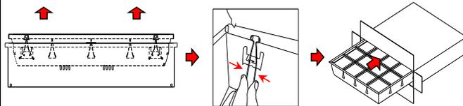
**Step 2:** Press the v-clip to release the louver from lamp frame and place it inside the box until the other installation processes are finished.
