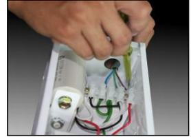
**Step 4:** Insert the supply cables into the transformer box then connect it to the provided connector.
