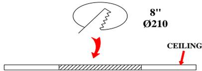
**Step 1:** Prepare hole at the ceiling according to fixture.
